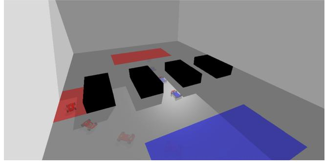
Fig. 3: Multi-step RCIP is applied in **Hallway Navigation**. The robot car (blue) and human car (red) are tasked with navigating to their respective goal states (large blue and red rectangles). The human car is constrained via its intent to pass through one of the five hallways (highlighted in red). The blue car does not observe the human’s intent during evaluation.
