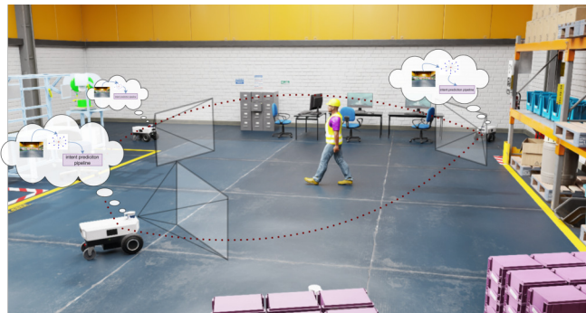
Fig. 1: Deployment of a multirobot system in Isaac Sim for human intent prediction. The robots create a graph representation for spatial understanding, incorporate information from the neighbors, and deploy a GRU for temporal understanding.
